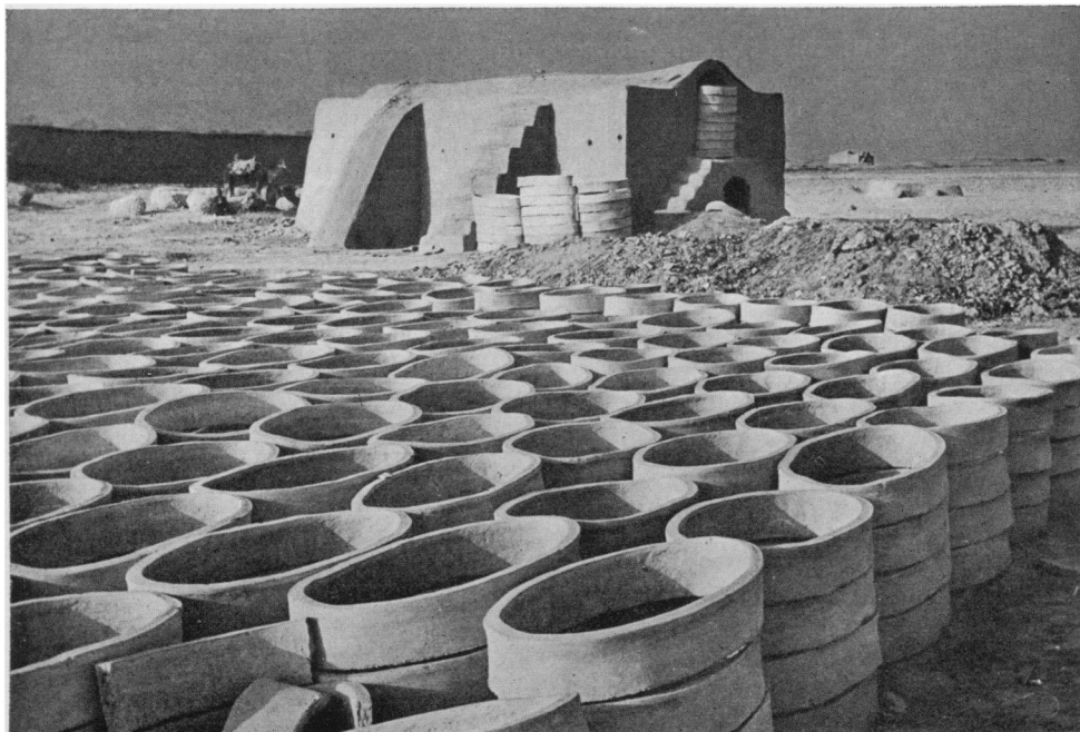
FIG. 3—Oval tiles, or nars , used to line the qanat tunnels. (Photograph courtesy of William E. Warne.)
